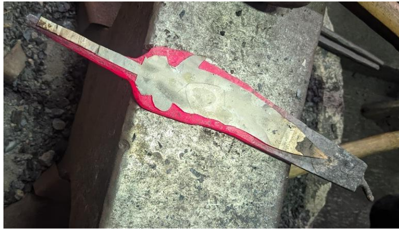
Figure 10. Sticking design model on to spearhead candidate.
