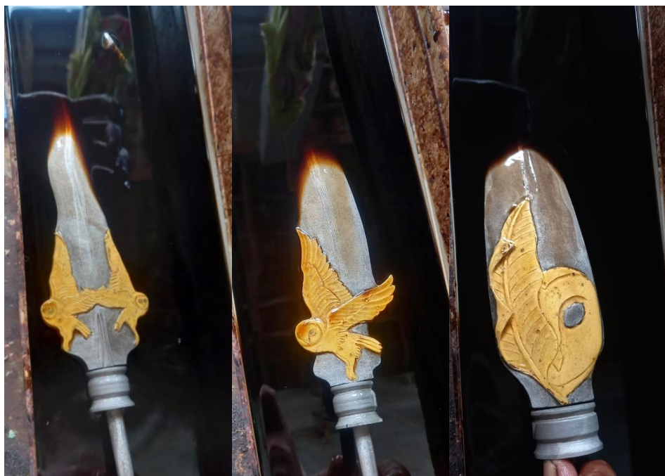
Figure 15. Black oxidizing process using arsenic acid, after gilding (gold electroplating).
