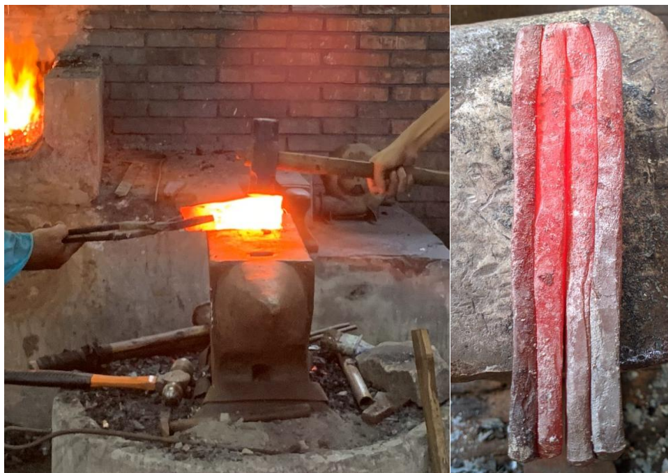
Figure 6. Pamor making. Forged iron and nickel.
