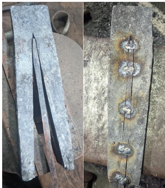
Figure 7. Inserting pamor in the center of iron.
