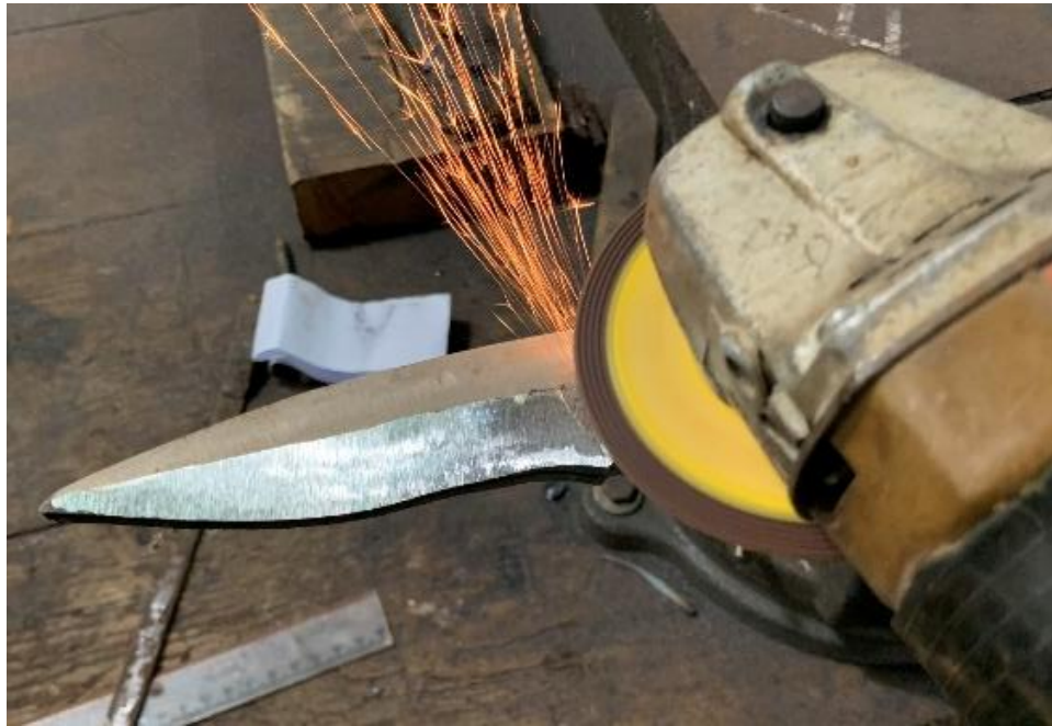
Figure 12. Shaping edges by grinding
